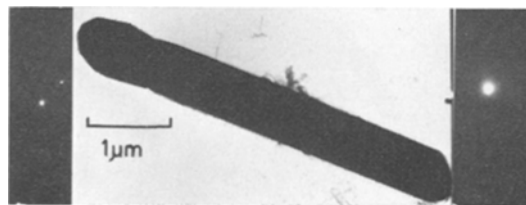
Figure 7 Spheroidization at the tip of a whisker extracted from a 20 vol % composite annealed for 500 h at 1200^\circ\text{C} .
